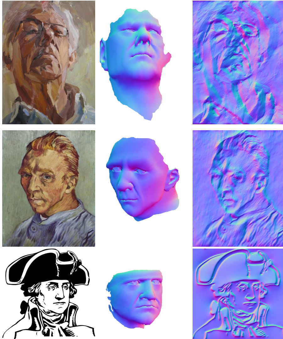
Figure 3.11: Examples of recovered normal maps from paintings and drawing. (left) Input image; (center) Normal map recovered using our method (all proxies derive from the same 3-D model); (right) Normal maps created using a commercial software (CRAZYBUMP, 2014).
